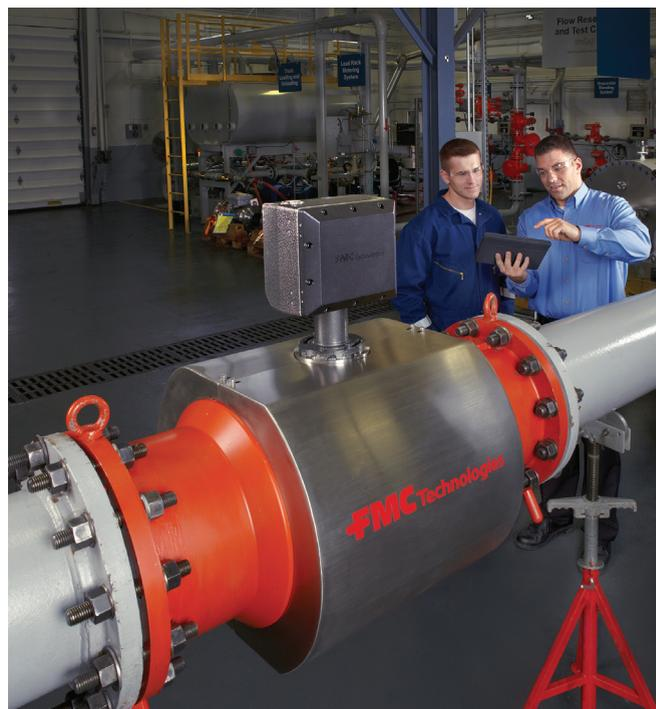
*To determine the velocity profile more accurately, custody-transfer ultrasonic flowmeters use multiple sets of transducers on chordal paths. The multiple chordal paths help in detecting whether the flow is laminar, transitional or turbulent. The number of paths, their location, and the algorithms that integrate the path velocities into an average velocity all contribute to the meter's accuracy.*
